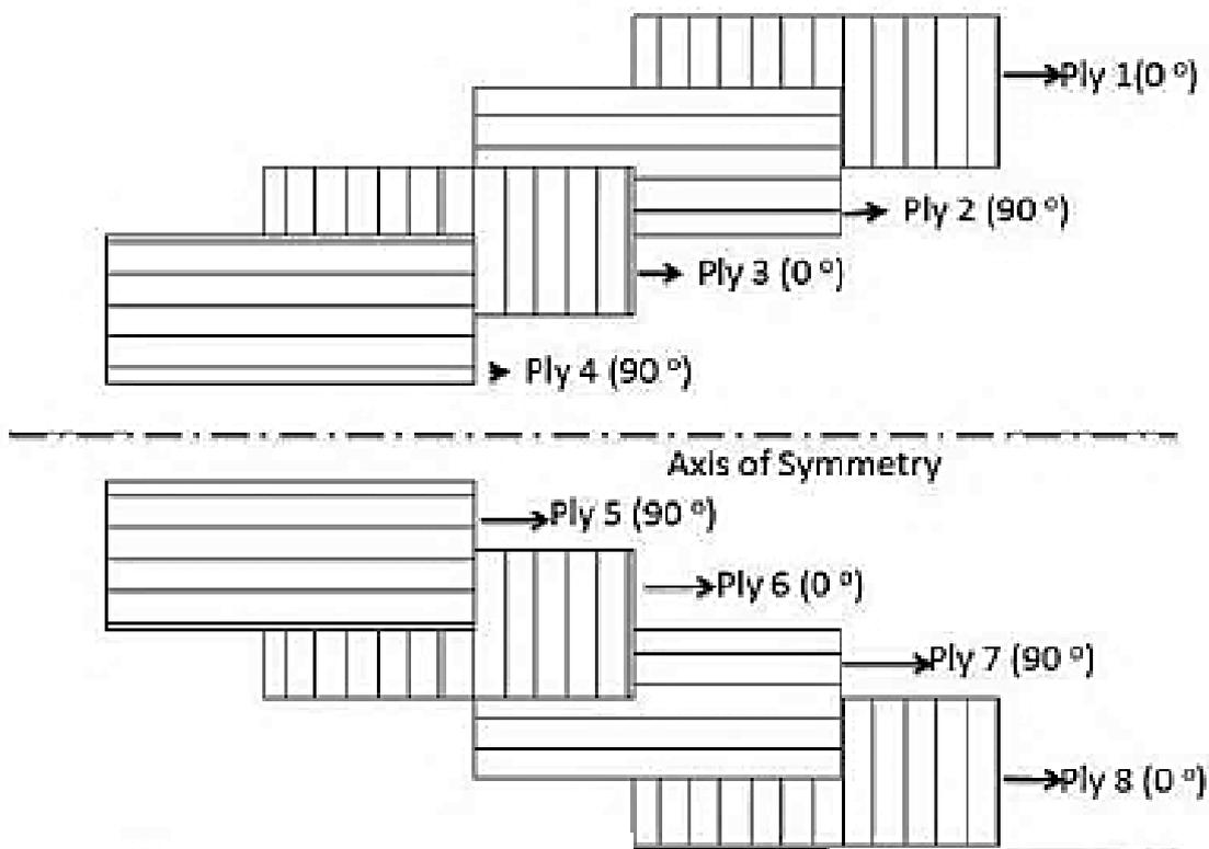
Figure 3. A Schematic sketch for different plies used in sample manufacture  $[0, 90]_2s$  (Mohammed et al., 2014)
