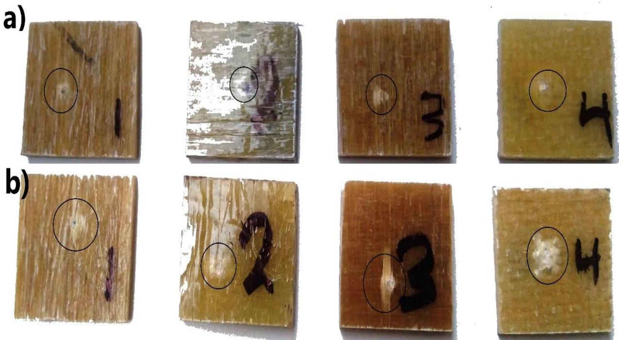
Figure 8. Damage surface depth through surface for: (1) [0]4s, (2) [0,90 ± 45] s, (3) [0,90] 2s, (4) Woven a) when h=1.5 m, m=1 kg, b) when h =1.5 m, m=2 kg
