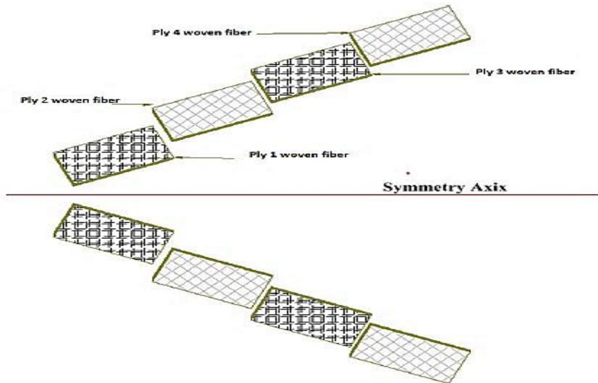
Figure 4. A schematic of the different woven plies used in sample manufacture (Abdellah et al., 2021)
