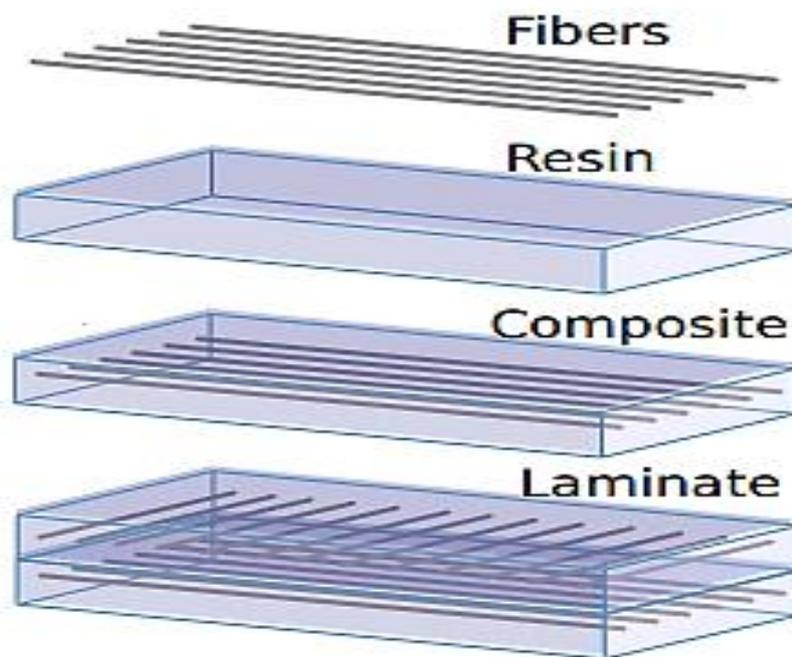
Figure 1. Schematic picture of a composite laminate (Jareteg et al., 2016)
