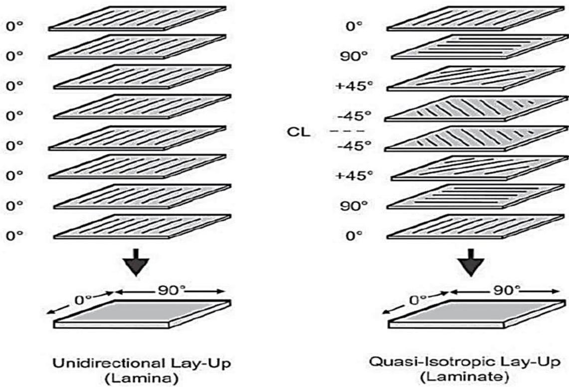
Figure 2. A Schematic sketch for different plies used in sample manufacture  $[0]_4s$  and  $[0,90 \pm 45]_s$  (W.J. Cantwell, 1991)
