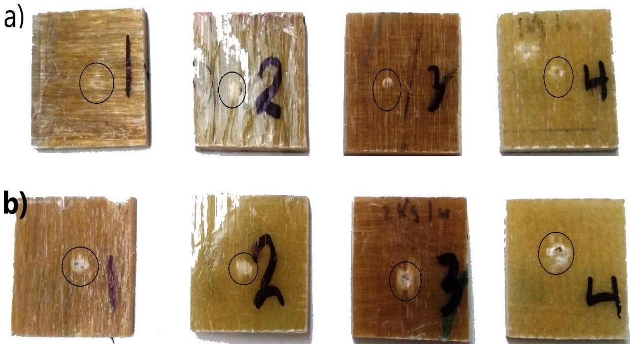
Figure 7. Damage surface depth through surface for: (1) [0]4s, (2) [0,90, ±45] s, (3) [0,90]2s, (4) Woven a) when h=0.1 m, m=1 kg, b) when h= 1 m, m=2 kg
