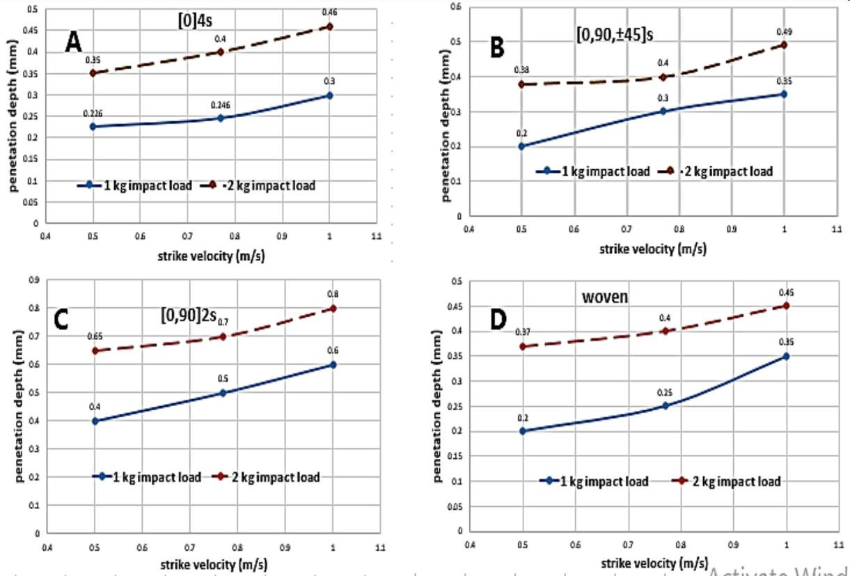
Figure 5. penetration of damage variation with impact strike velocity for A) [0]4s, B) [0,90 ± 45] s, C) [0,90]2s, D) woven
