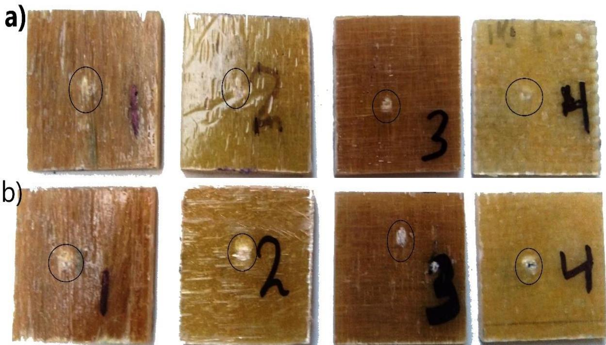
Figure 6. Damage surface depth through surface for: (1) [0]4s, (2) [0,90 ± 45] s, (3) [0,90] 2s, (4) Woven a) when h=0.5 m and m=1 kg, b) when h=0.5 m and m=2 kg
