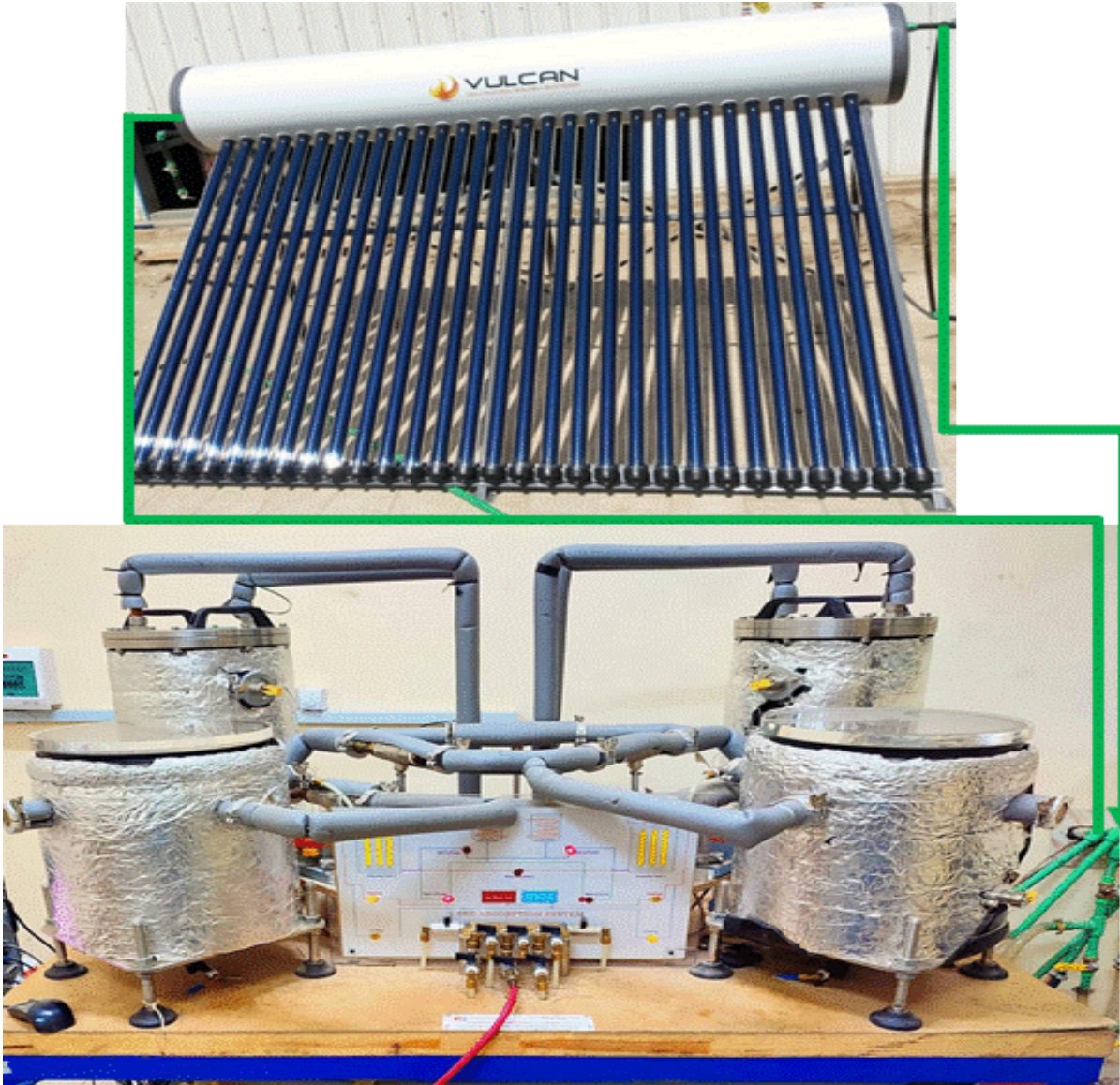
Figure 1. Photo of experimental adsorption desalination system
