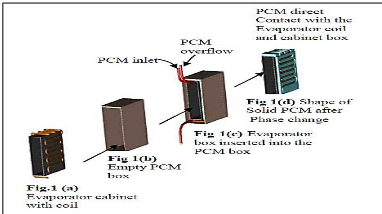
Figure 4. The arrangement of the PCM based evaporator. (Khan et al., 2011)
