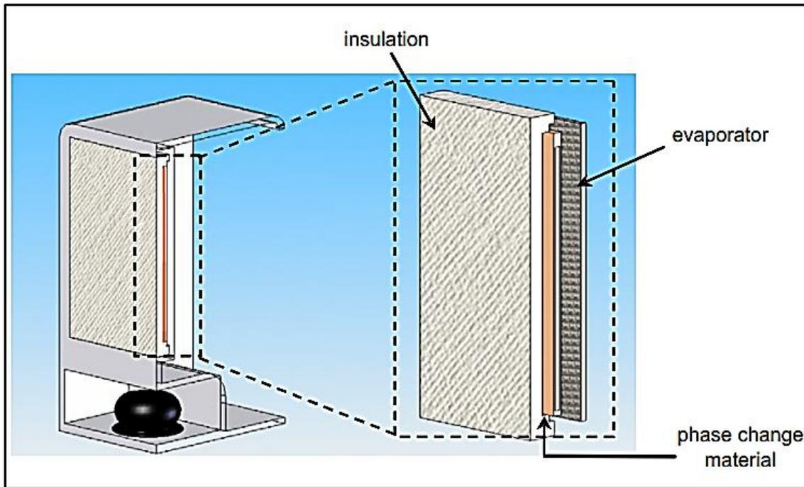
Figure 2. Construction of the PCM along with evaporator side. (Azzouz et al., 2008)
