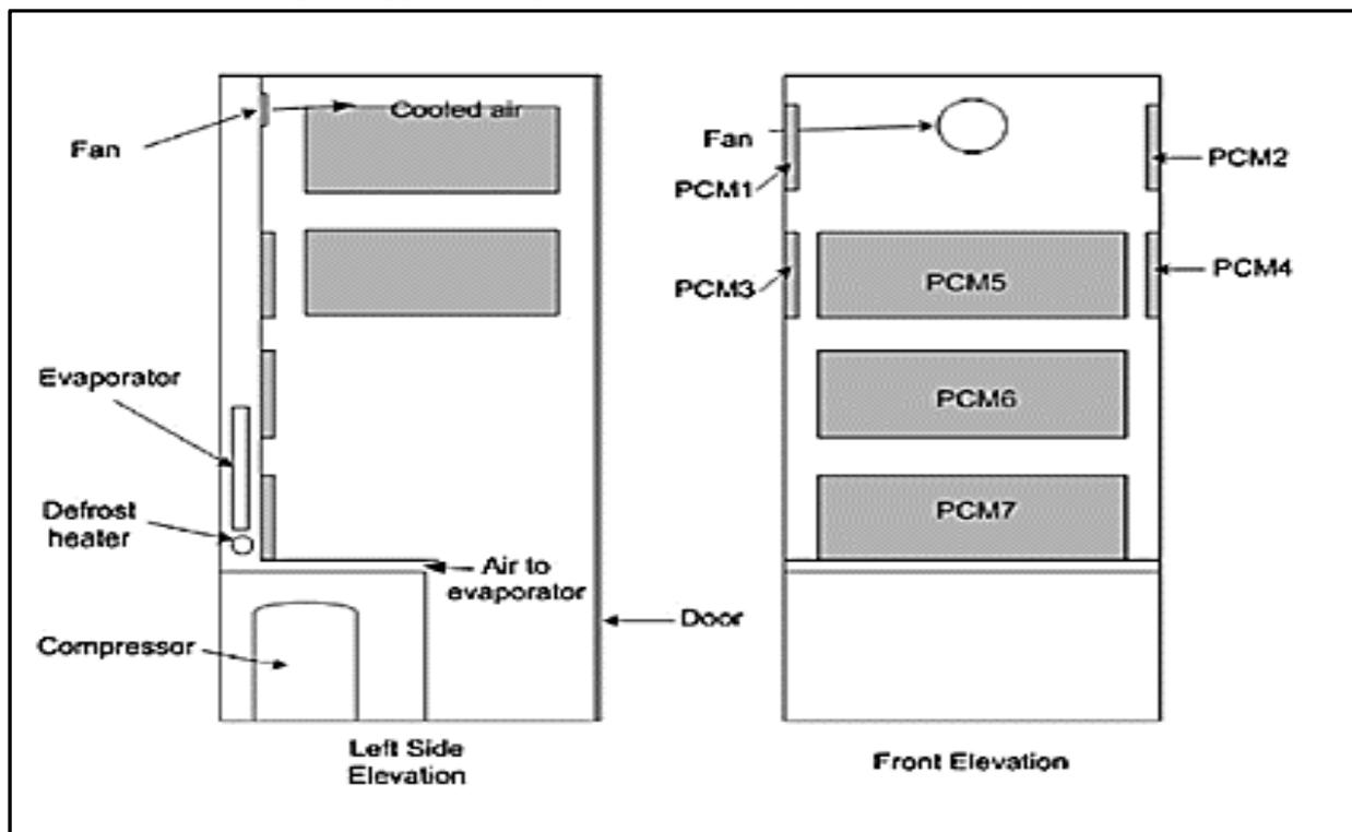
Figure 3. Schematic of the freezer showing positions of the evaporator, defrost heater, and placement of the panels (Gin et al., 2010).
